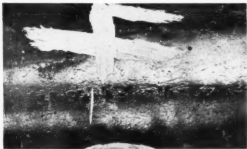
Fig. 9—Seam in a length of 3 1/2-in.-o.d., 9.30-lb., N-80 tubing which did not fail at 15,000-psi. pressure.
